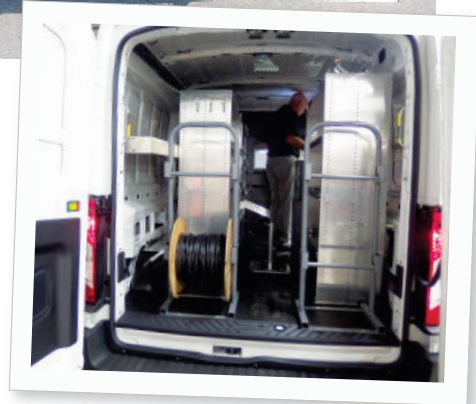
Time Warner Cable is creating a more usable space in the rear of its full-size Transit Vans, and with the medium-height roof, workers are able to stand and easily access equipment. The company is also standardizing the upfits where possible.
